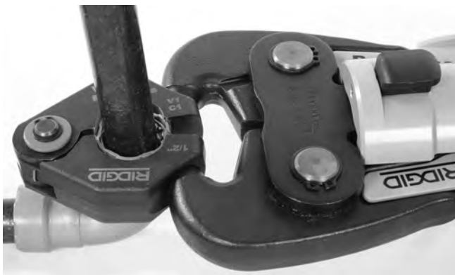
Figure 12 – Attaching Actuator to Press Ring
